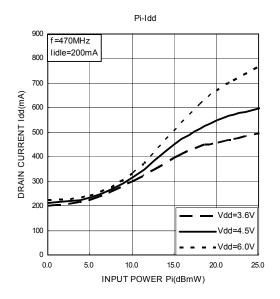
Note 4: These are only typical curves and devices are not necessarily guaranteed at these curves.
